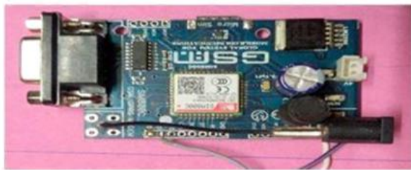
Fig 5. GSM Module interfacing with arduino.
